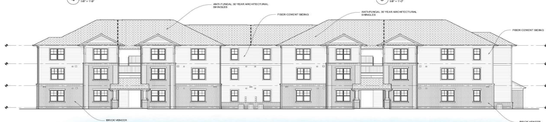
2 BUILDING 100 - REAR ELEVATION 1/8" = 1'-0"
