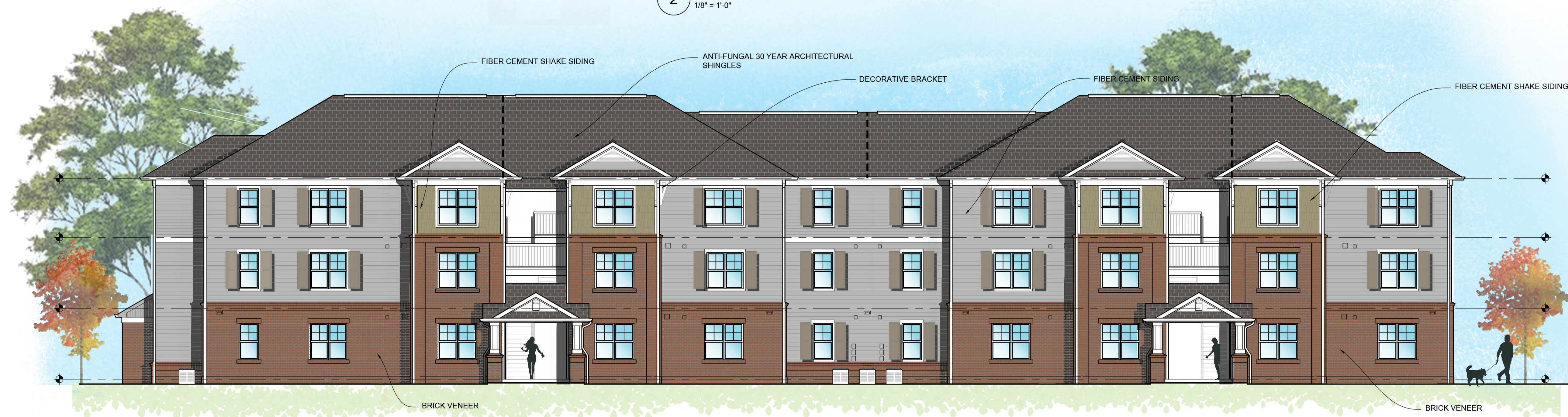
1 BUILDING 100 - FRONT ELEVATIONS ( PARKING LOT SIDE ) 1/8" = 1'-0"
